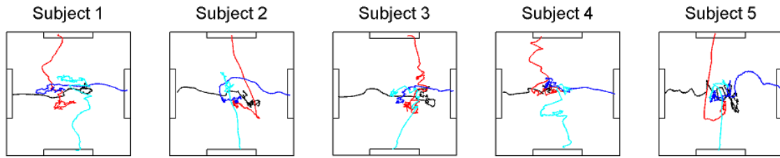
Fig. 3.6. Mean brain-controlled cursor paths. Each colored path is the mean of the length-normalized trials for a single direction (left, top, right, or bottom) across all trials of all runs for a subject. Trials in which subjects did not acquire the target within 15 s were not included in the analysis. The workspace dimensions were 30 x 30 cm.
